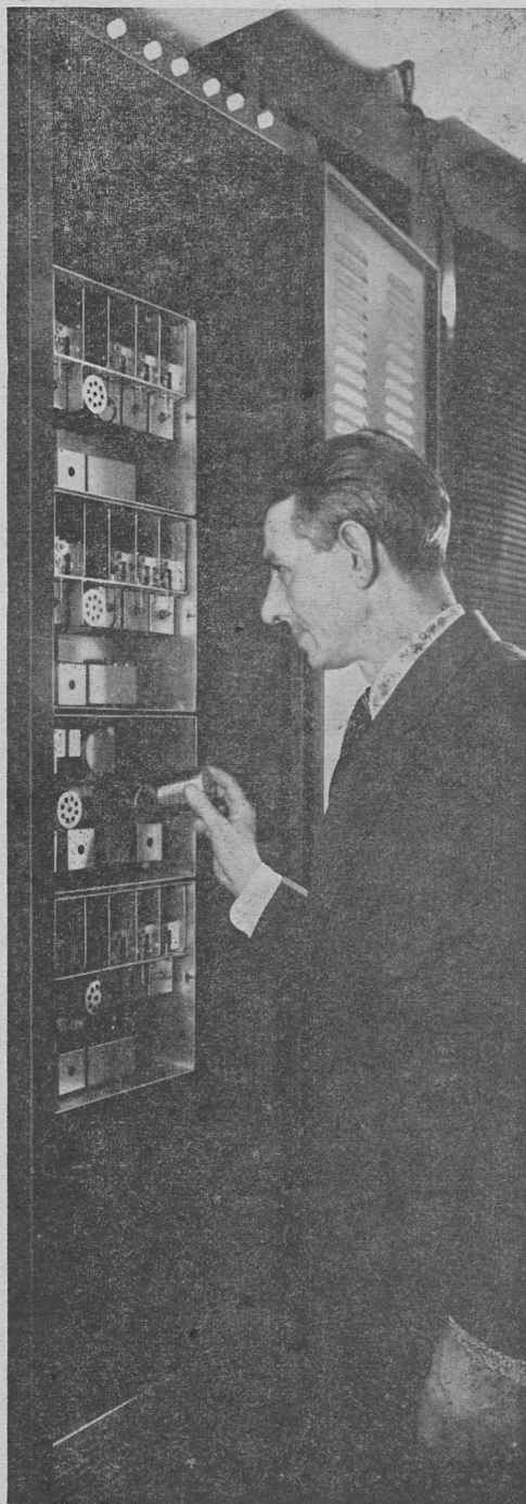
Fig. 5—In the intermediate-frequency amplifier, shown undergoing inspection by F. Stevens, Radio Technician of the Waldorf, the power of the signal is increased a hundred thousand million fold
